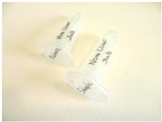
1.5mL or 2mL reaction annotated tubes (Eppendorf type or flat cap/screw cap tubes)
